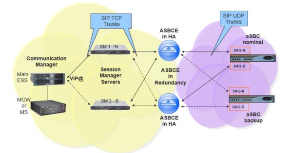
ASBCE in Redundancy mode deployment (Geographic-redundant deployment) is a multiple ASBCE deployment. ASBCE in redundancy can be deployed in the HA (High Availability) or non-HA mode. ASBCEs in redundancy are available at the same time and the calls can be routed over them depending on the dialplan on ACM/SM or AS (Application Server).
