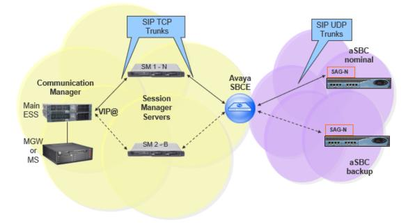
When the Survivable Core Server (ESS) is implemented in the architecture and the communication to the Primary Controller (main ACM server) is lost then all the IP telephones and Media Gateways and Media Servers register to a Survivable Core Server (ESS).
