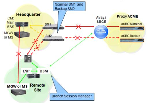
When communication from Remote Site to the Primary Controller (main ACM server) and Survivable Core Server (ESS) is lost then the Remote Site's IP telephones and Media Gateways and Media Servers register to the Survivable Remote Server (LSP) and SIP telephones register to the Branch Session Manager (BSM).
